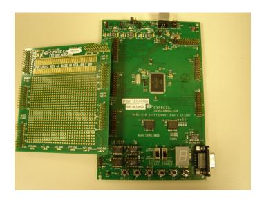
The development kits for the MoBL-USB FX2LP18(TM) family provide complete hardware and software solutions for accelerating the firmware and device driver development for all the products in the family. The development kits use the actual silicon for the entire development. Cypress's software utilities and example firmware allow the user to generate USB traffic in hours, not weeks!
