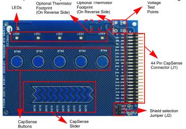
The module consists of five CapSense buttons, one linear slider (with ten sensors), and five LEDs. These are interfaced to the CapSense controller board via 44 pin receptacle connector (J1). A three pin jumper (J2) is provided for selection between shield electrode and ground. The board also incorporates an optional I2C EEPROM and thermistor that are not populated by default.
