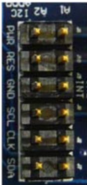
Figure 2-3. Six Jumpers Available on Board
