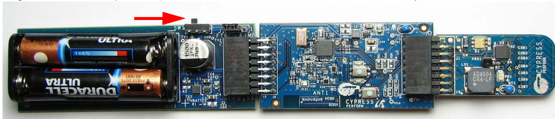
Figure 3-9. RF Expansion Board into the 2x AAA Alkaline Cell Battery and MultiFunction Board
