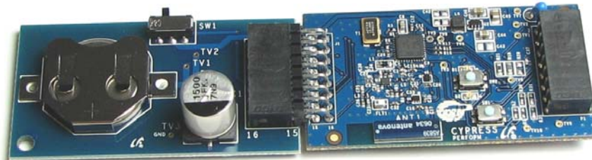
Figure 3-3. RF Expansion Board into the CR-2032 Coin Cell Battery
