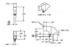
Bright•Pipes<sup>™</sup> Optical Lightpipes produce bright, even indication based on optical ray tracing. They conveniently and economically conduct light from SMT LEDs through angles and distances to a viewable front lense surface in order to provide an attractive, bright and even indication of equipment of function status with a minimal attenuation of light output through the optical fibers that join the base, at the LED light source, to the lens front.
