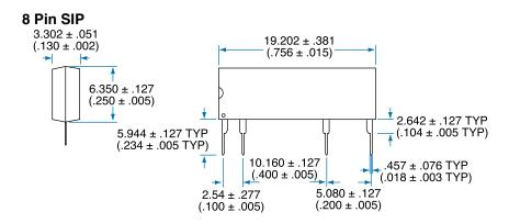
**Note:**1. Pin location tolerances are non-accumulative.
