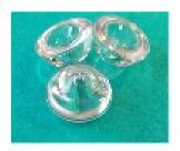
120 deg bubble optic for even wide area light output use optic on it's own with the Rebel and Cree Xp and with a holder for the K2 and SSC P4. Circular and 1.5 mm diameter.
