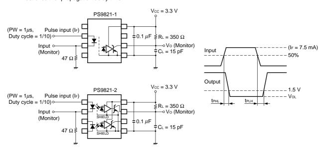
$\textbf{Remark} \quad \textbf{C} \textbf{$\llcorner$ includes probe and stray wiring capacitance}.$
