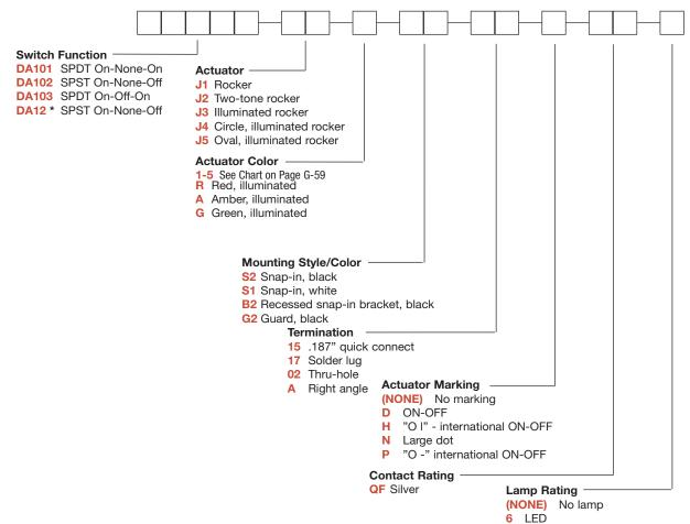
\* DA12 — for switches with both marking and illumination
