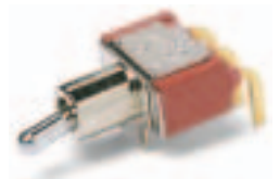
7101MD9ABE Horizontal Actuation SPDT
