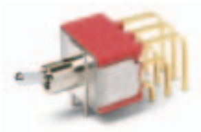
7301MD9AV2BE Vertical Actuation 3PDT
