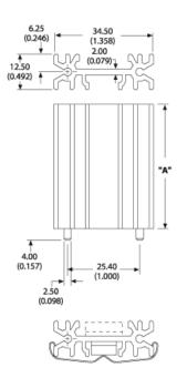
X Dim: 12.70 (0.500) | Y Dim: 1.00 (0.040) | Z Dim: 3.0 (0.118)
