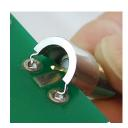
V-Bite<sup>®</sup> Edge-Mount connectors are fast and simple to install. Simply place the connector at a 45-degree angle to the PCB. Insert the PCB into the notched opening and push down onto the connector to seat it firmly in place.
