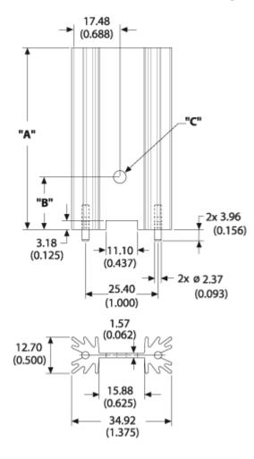
A Dim 25.40 B Dim 18.29 C Dim 3.18
