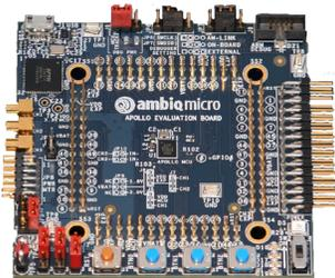
The Apollo Evaluation Board, or EVB, is the center of your low power computing system. The EVB includes a APOLLO512-KBR, which has an ARM M4F core, 512KB of Flash memory and 64KB of SRAM in a 64-ball BGA package. All of the I/O and peripheral functions are routed to easy to access 0.10” headers making prototyping painless.
