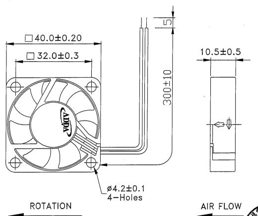
LEAD WIRES: UL 1007, AWG26, L = 300 +/- 10 mm Red = positive; Black = negative.
