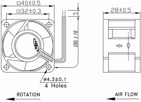
LEAD WIRES: UL 1007, AWG26, L = 295 +/- 10 mm Red = positive; Black = negative.
